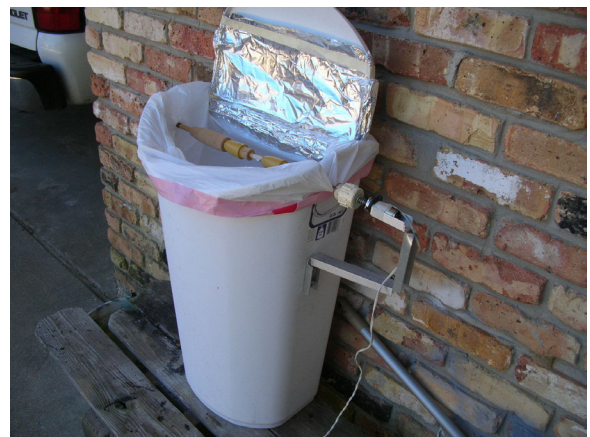
Fig 04 A Containment System Compressed Air Spraying
