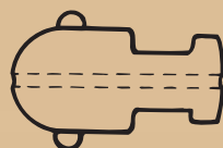
Fishing line threads through 3/32" diameter hole
