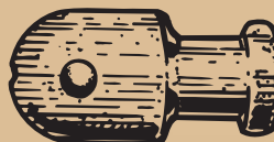
Fishing line threads through 3/32" diameter hole
